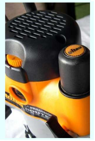
Now remove the screw (30) and the micro adjust knob (31).
