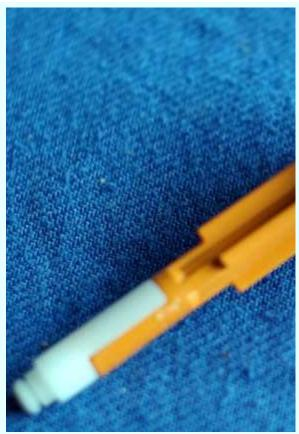
One of the fiddly parts of this process is to re-assemble the plunge selector rear section (white), complete with its spring, back onto the orange plunge selector.
