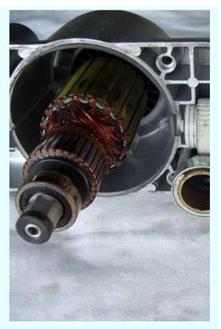
Now is the time for a good clean, blow out with an airline, light lubrication, etc.
